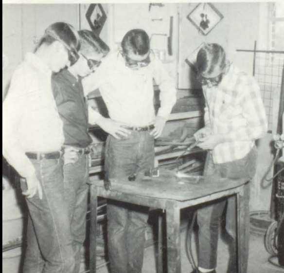
Second-year boys are learning to fuse and braze weld with the oxyacetylene welder.
